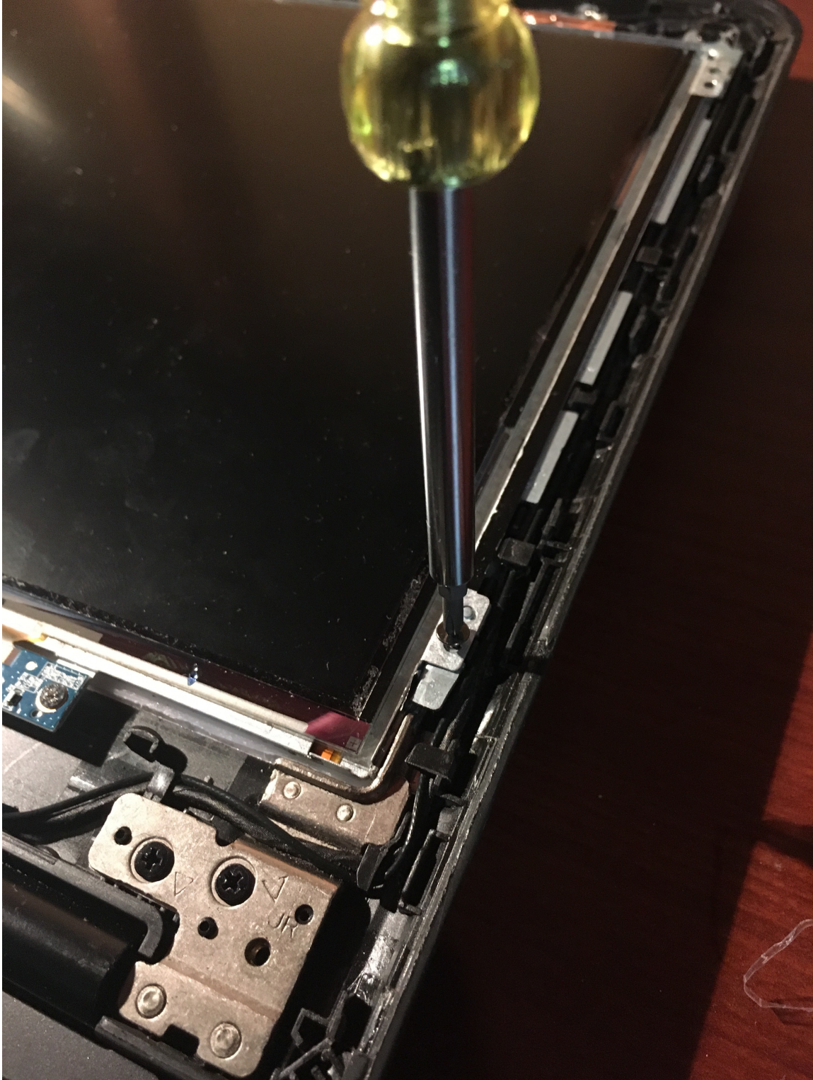
unscrew the sides holding the display to the case
