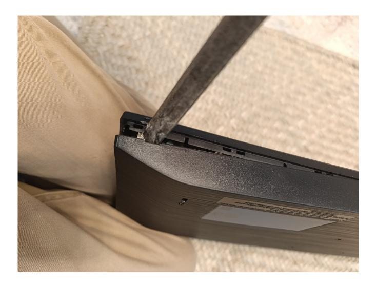
then find a suitable entry space in a bottom corner and start to remove the bezel carefully by a twisting action, do not to insert the tool edge too far in or you may permanently damage the components, make your way carefully little by little in one direction until you hear a snap sound and cover or bezel starts coming apart.
