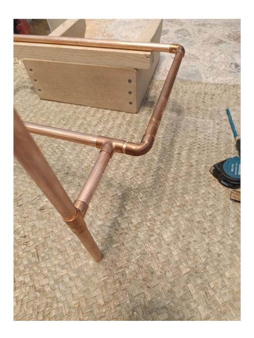
when the frame is fully cured, then its time to glue the base, glue the angles in the same way and measure you have the correct square angle by placing some square thing and aligning it with the frame, and leave this to cure for the appropriate time before moving to the next step.
