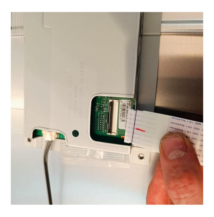
Remove one and then the other, one has to be pressed sideways to get it out, the other has a latch, do it carefully and slowly, if you are not careful you will damage a microscopic pin and the monitor will not be usable
