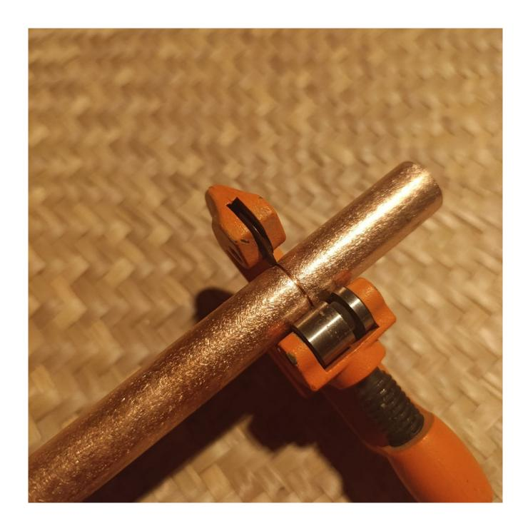
Take this outer siamenter measurement and multiply it by .75 then subtract this number by the absolute length of each side of the panel, and cut the copper pipes exactly to each of the measurements with the pipe cutter.
