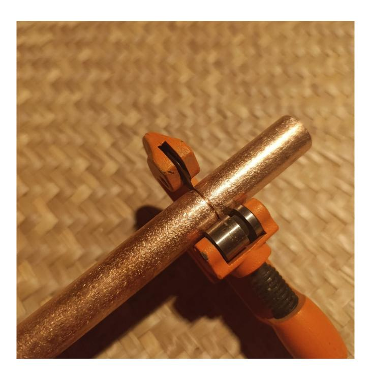
carefully remove the panel and put it in a safe place, the take that copper tube and cut it in the markings
