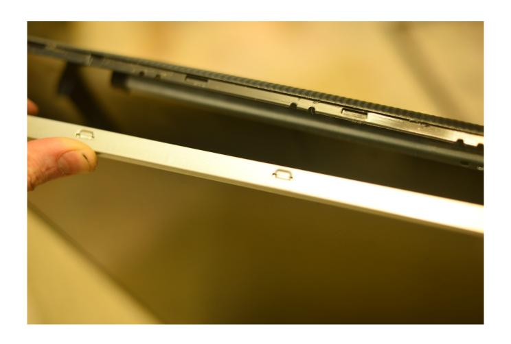
in case your panel does not come out effortlessly when placed faced down, carefully turn the panel to the side and find any side screws and unscrew them
