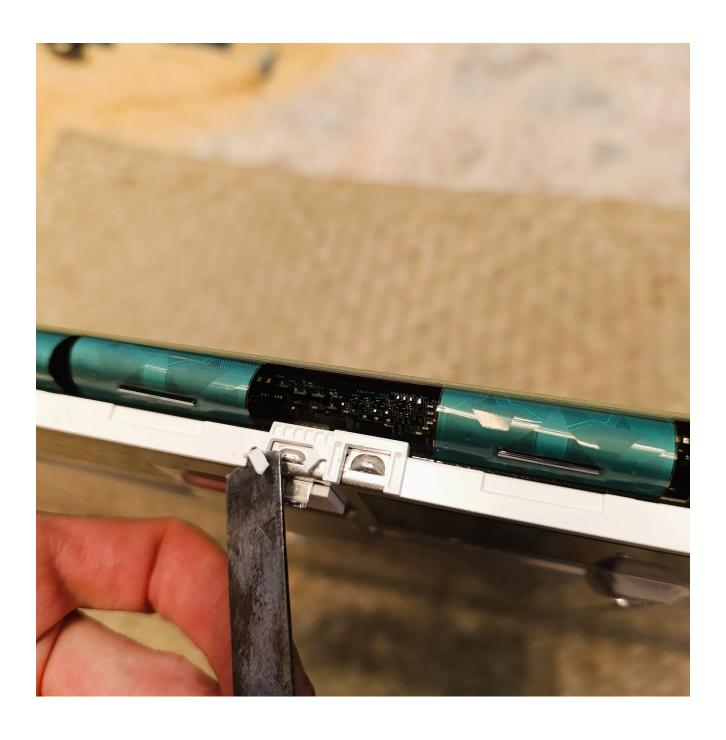
you may also find these locks holding a frame in place, they are easy to unlatch, and at the very last do the bottom side with the ribbon connectors with the utmost attention
