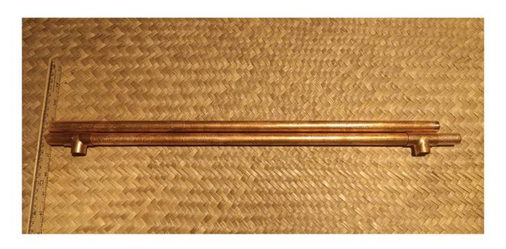
take both bottom and top tube and put them together side by side, nicely aligned, then mark where the extra length is
