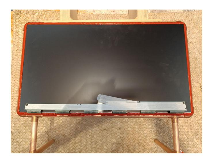
put some masking tape to hold the card to the panel, do this only in a small edge so its easy to take off, otherwise you will have trouble taking it out, and might damage the ribbon cables in the process, any mistake that pulls these ribbons too much will not reparable, and you will have throw the panel in the trash, so take your time and do it slowly and follow the process verbatim. Put the silicon under the ribbon cables, putting silicon here is very important so the panel holds tight.
