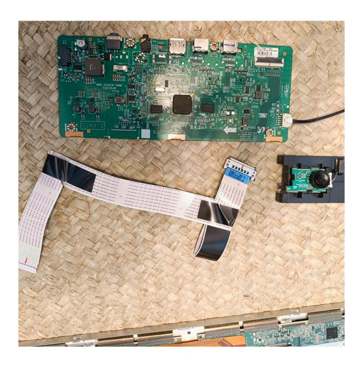
and you will be able to remove these components: an electronic board with the ports, a ribbon cable and maybe a menu button, and if you have an internal power supply that as well.
