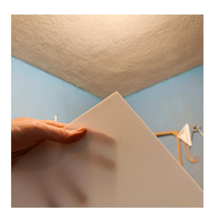
you will also find a hard acrylic sheet, either transparent, milky white, or grated, save this, and discard the last completely white sheet than you cant see through. If you will find a milky white hard acrylic sheet, then these are the best for making incandescent bulb backlit monitors and there is no need for doing anything further with these because are ready.
