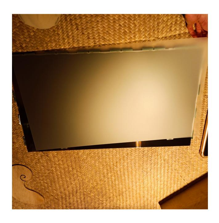
and put them directly into the back of the LCD panel, with the matte side facing up
