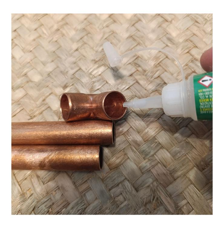
Now that you have the correct measurements, its time to glue the copper frame together, you will need some some glue, glue both inside the angles and outside the tube
