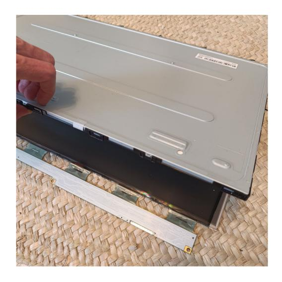
In some monitors there is no need to remove much more and the panel will just come out when placed faced down starting from the bottom, there may be a little glue holding the ribbon and card in place, but that's it. But be especially careful with the panel edges, as there may be some sticky tape holding it in place, if it does not come out effortlessly find the tape and carefully remove it, always watch the edges, if they are chipped the panel is gone.
