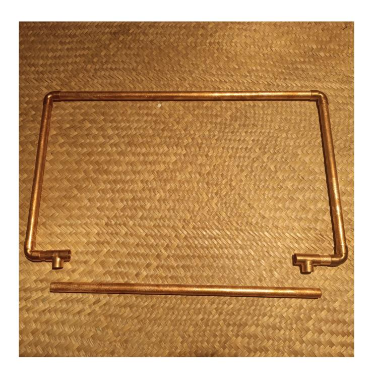
after this bottom tube cut, when you put the frame back with the "T" joints, it should look something like this, as you can see it does not fit like before, so we need to cut the top tube
