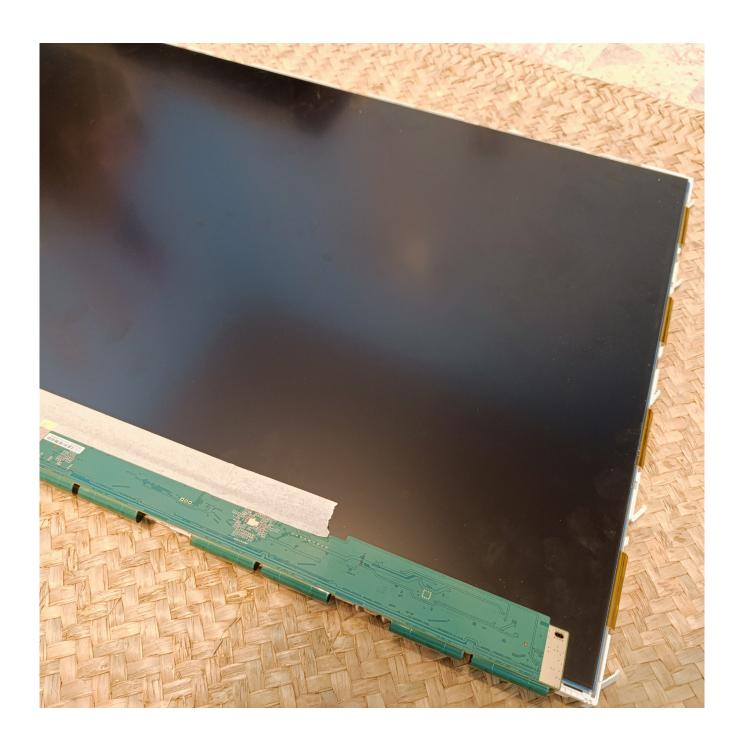
place the panel in a clean safe place face down, with utmost attention to the ribbon cables to not touch them too much, make sure there are no screws or anything in the space you will place the panel, and remove the rest of filters
